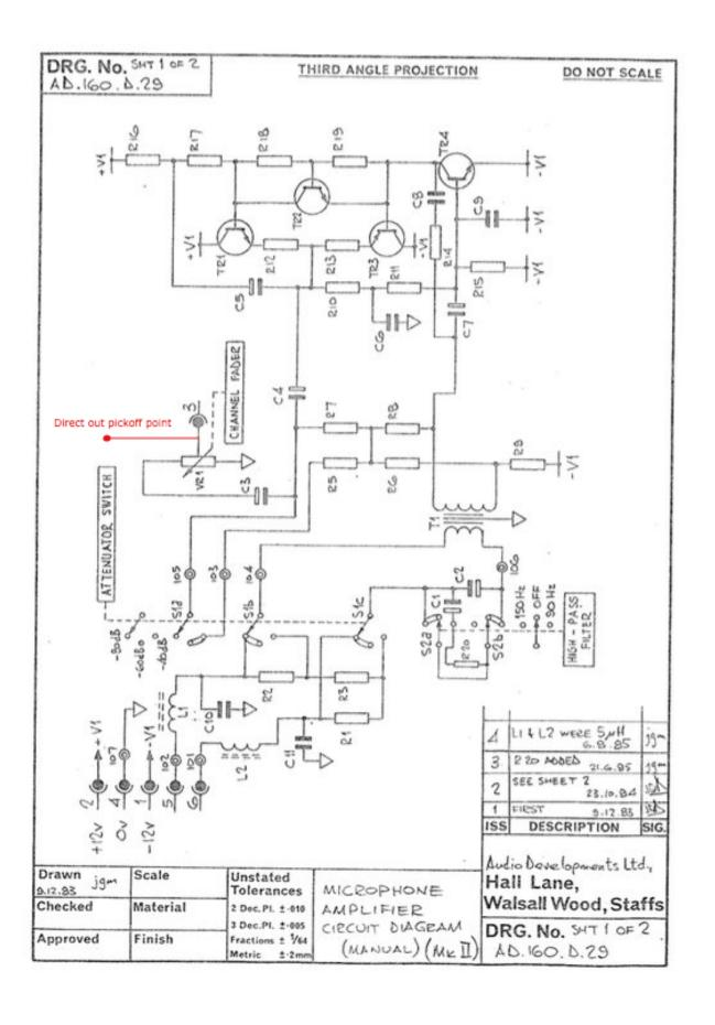
Step 2- Change the output XLR conector 3pin for an XLR 7pin. You can use this conector to send out the chanel 1, 2, 3 direct outs and the balanced mix bus.
